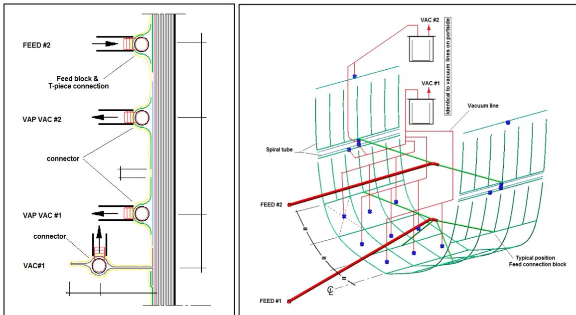
**Figure 5:** Principle of the 2-step continuous bag & reinforcement method. Layout of membrane material, vacuum connections and resin inlets shown at the left. At the right, the setup for a full scale infusion trial is shown.
