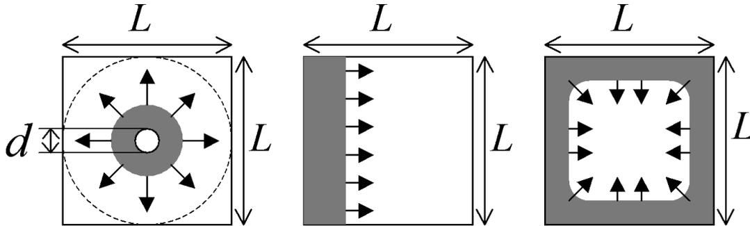
**Figure 3:** Three different injection strategies for a square plate with dimensions LxL. From left to right: point (slow to fast) injection (inlet diameter d), edge injection and peripheral injection.
