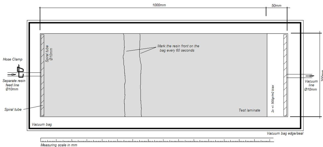
**Figure 2:** Standardized strip injection test for permeability measurement.
