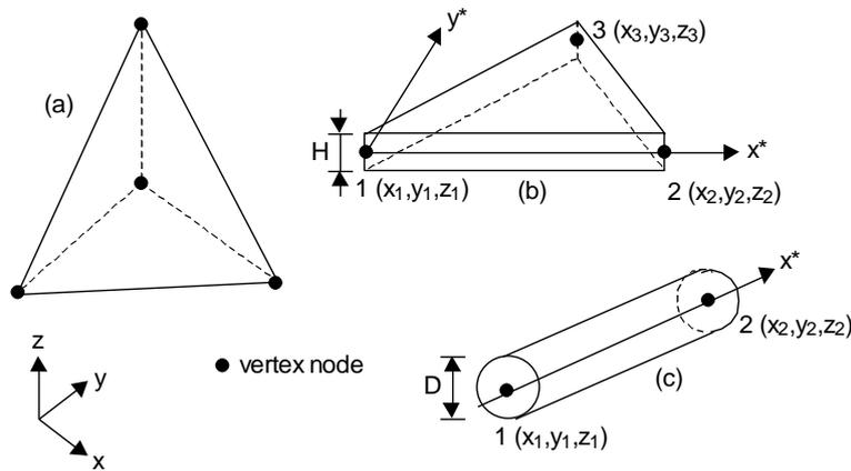
**Figure 1:** Basic element types for the unified GHS/RTM formulation, (a) 3D linear tetrahedron (Darcy flow only), (b) 2D linear triangular shell and (c) 1D linear runner (tube); where  $x^*$  and  $y^*$  denote the local co-ordinates and  $(x_i, y_i, z_i)$  the global co-ordinates.
