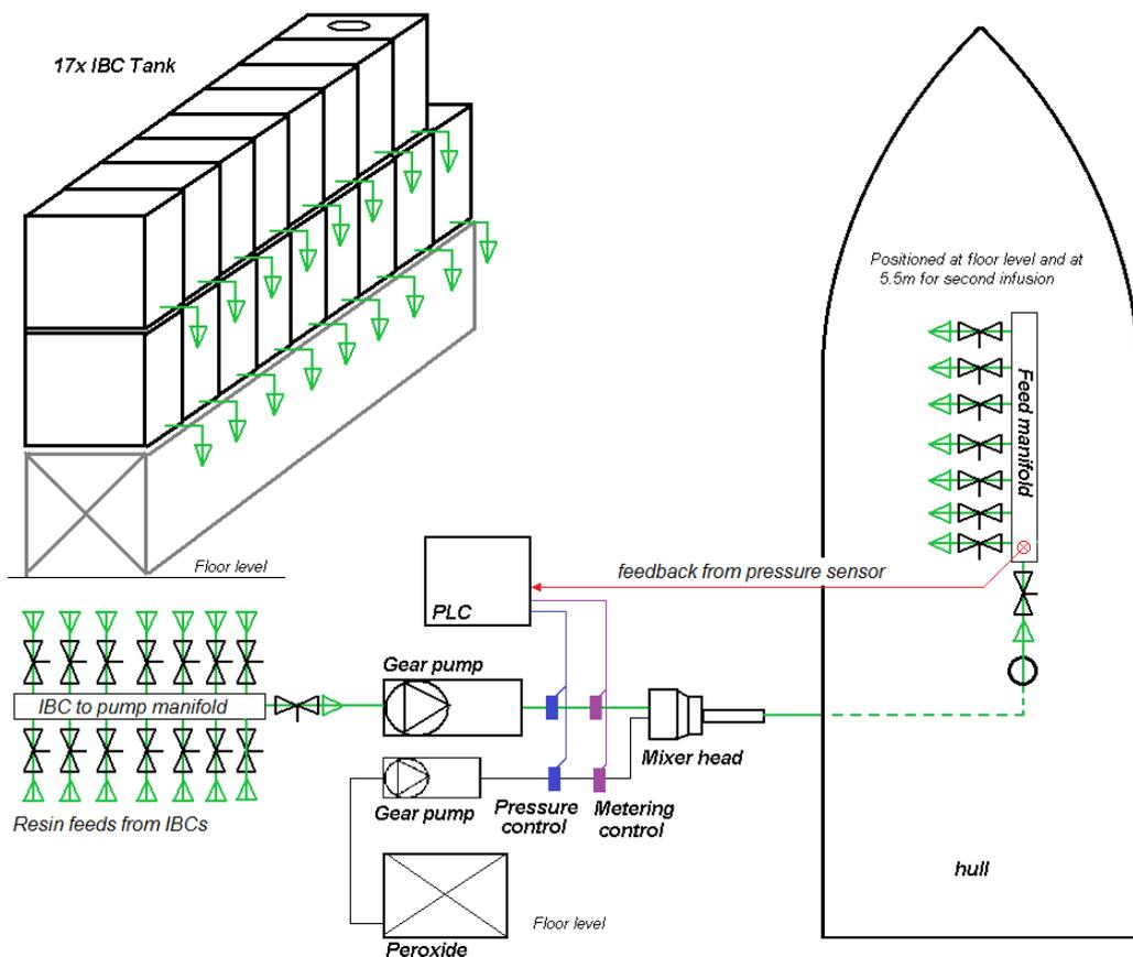
**Figure 6:** Schematic overview of the 2KM degassing and mixing equipment. Degassing was done prior to injection in a separate step. During injection, the mixing pump output was controlled by a pressure sensor located on the feed manifold, close to the bag to compensate for pressure losses in the long (30 meter) feeding tubes while guarding the vacuum level under the bag.
